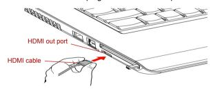
Figure 4-13 Connecting the HDMI out port
